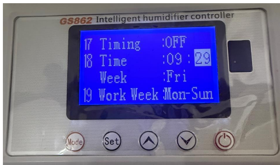
Figure 8-6 Timing, controller clock and Work Week settings
