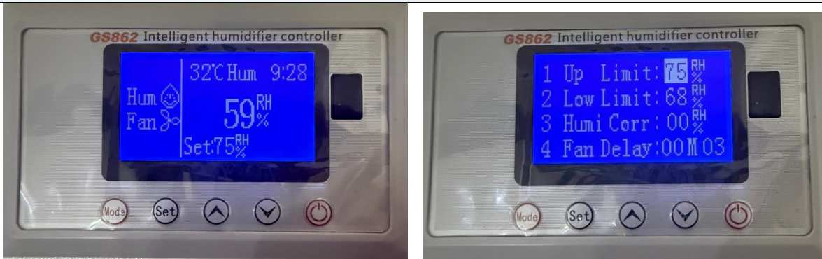
Figure 8-3 Humidity mode main screen and parameters 1-4
