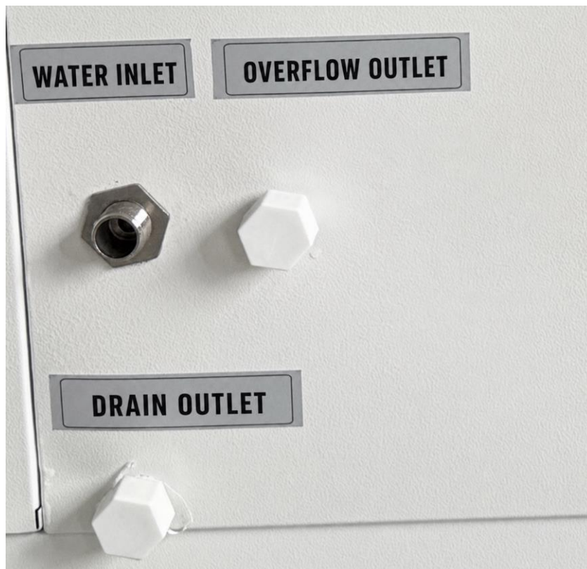
Figure 7-2 Water inlet, overflow outlet and drain outlet
