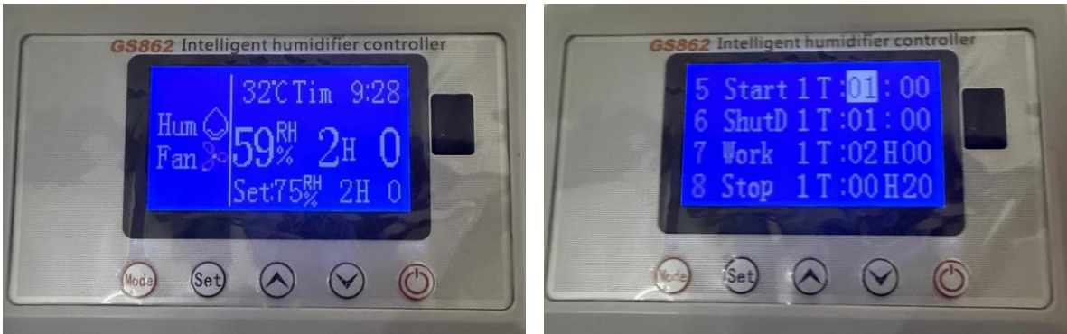
Figure 8-4 Timer mode main screen and period 1 settings
