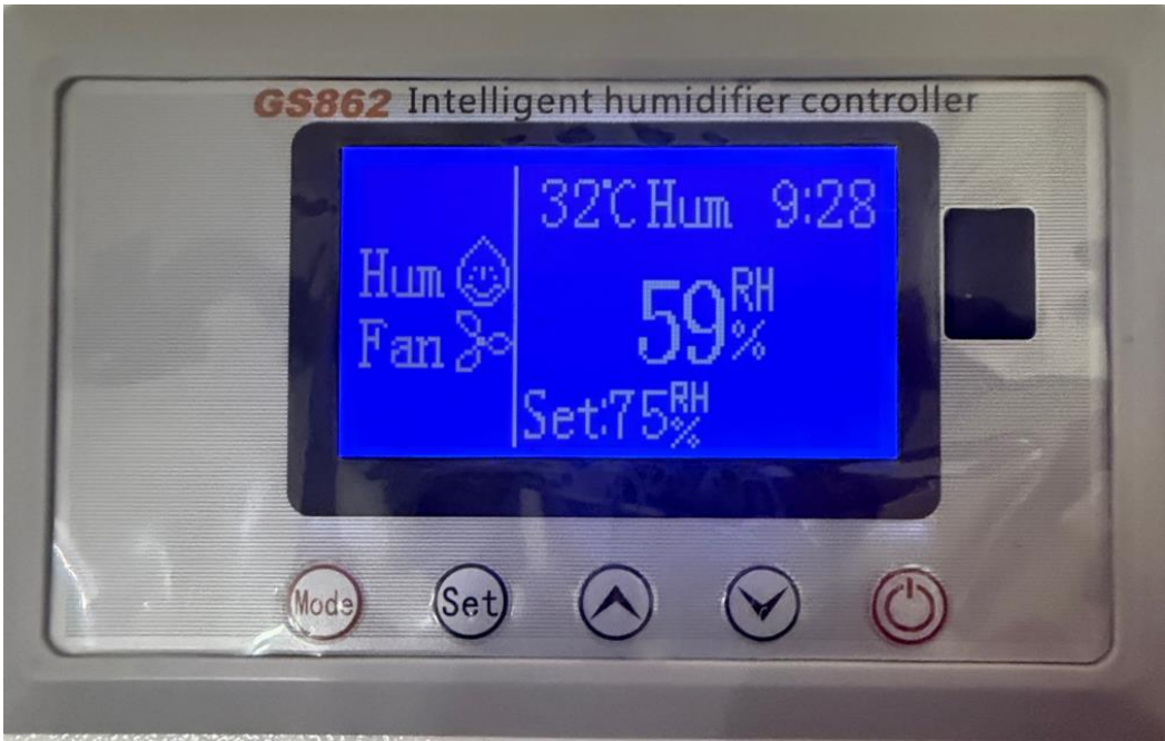
Figure 8-1 GS862 controller front panel and button layout
