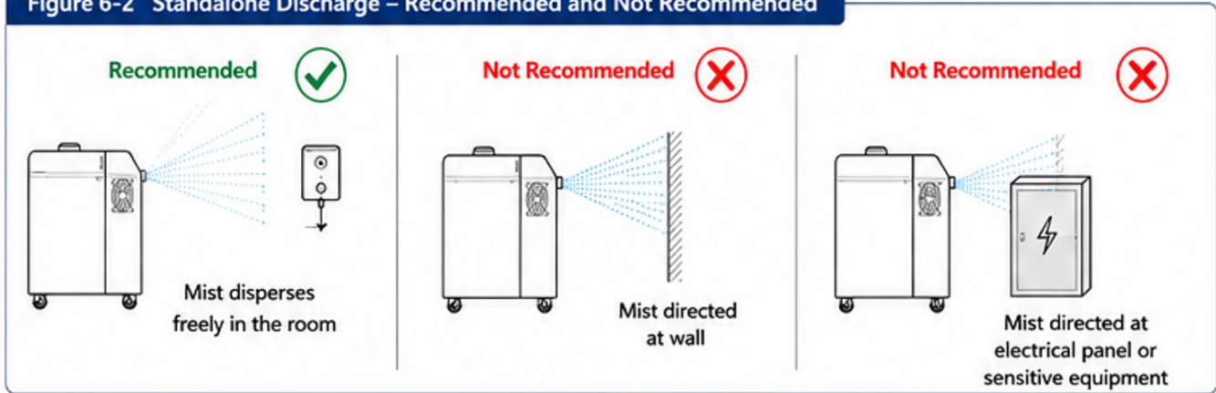
Figure 6-2 Standalone Discharge – Recommended and Not Recommended
